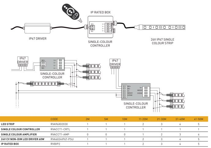
Note: Controller and amplifier only required for white flexi-strip that is to be dimmed
