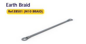
The Speedway Earth Bonding Strap (EBSo1) is designed for use in installations where an additional means of earthing or electrical bonding is specified. The Speedway Earth Bonding Strap comprises of a 16mm<sup>2</sup> tinned copper braid crimped into M10 tinned copper end connectors. The Speedway Earth Bonding Strap is common to Speedway SW4, SW5, & SW6.
