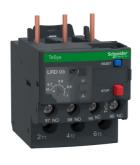
Thermal overload relay, TeSys Deca, 690VAC, 0.63 to 1A, 1NO+1NC, class 10A, screw clamp
