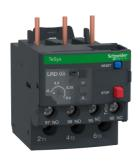
Thermal overload relay, TeSys Deca, 690VAC, 0.25 to 0.4A, 1NO+1NC, class 10A, screw clamp
